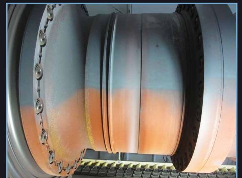
A TURBINE SHAFT DURING THE DRY ICE BLASTING PROCESS
