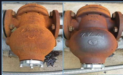
RUST EASILY REMOVED FROM A VALVE WITH DRY ICE BLASTING
