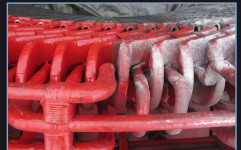
THE DIFFERENCE OF AN ELECTRICAL STATOR BEFORE (RIGHT) AND AFTER (LEFT) DRY ICE CLEANING
