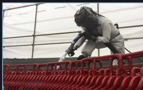
A MEMBER OF THE POLAR ICETECH TEAM DRY ICE CLEANING AN ELECTRICAL STATOR
